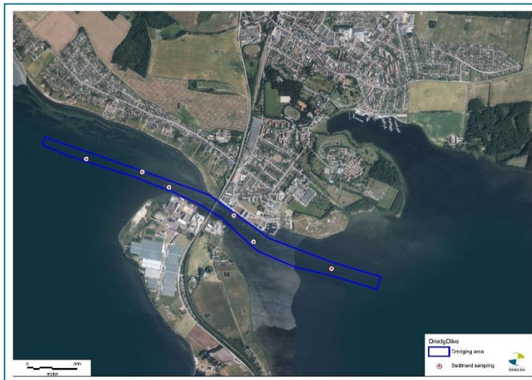
Figure 16: Dredging area and sediment sample locations.
